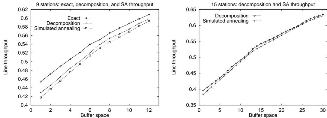
Figure 4: Computed throughput of simulated annealing compared with full and reduced enumerations for 9 stations (left); compared with reduced enumeration for 15 stations (right).
