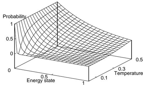
Figure 2: Probability distribution  $w \sim \exp(\frac{-E}{kT})$  of energy states according to temperature.
