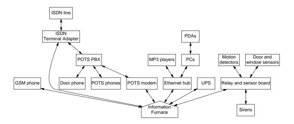
Figure 3: Information furnace connection diagram.
