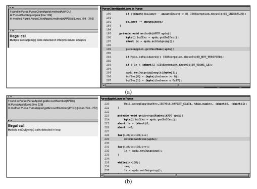
**Figure 5.** Illegal use of setOutgoing() detected (a) in interprocedural analysis and (b) within a loop via call to another method
