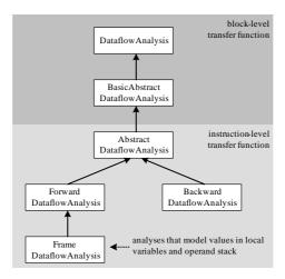
Figure 6. FindBugs base classes for dataflow analyses
