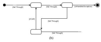
**Figure 3.** CFG patterns with basic blocks corresponding to (a) for/while and (b) do . . . while loop
