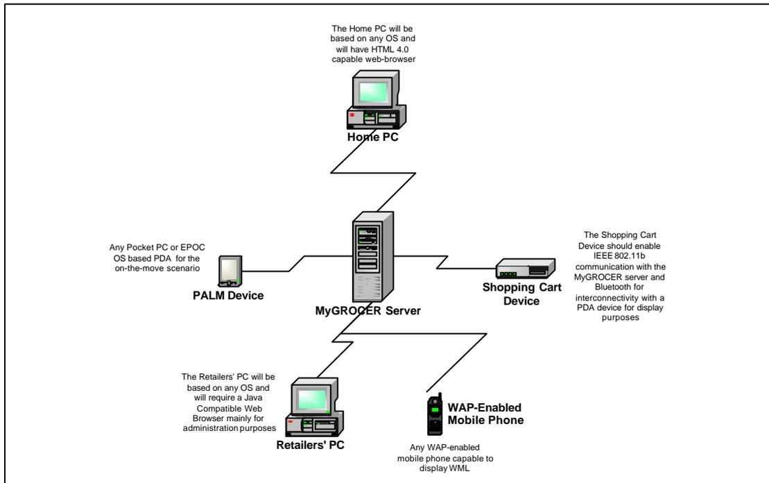
**Figure 2: Integration of MyGROCER with different devices**
